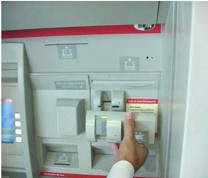
Card copying equipment being installed on front of a cash machine. This gadget records your card details.
