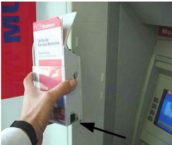
Card copying equipment being installed on front of a cash machine. This gadget records your card details.
